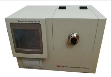
For power system, industrial and mining enterprises, there have a lot of oil filled electrical equipment, so the acid value of the transformer oil and turbine oil is regular inspection item which need to be measured.
